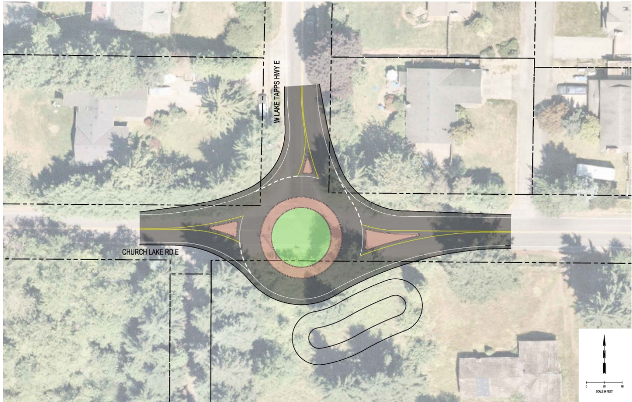
Figure 9. Church Lake Road E at W Tapps Highway - Roundabout Alternative
