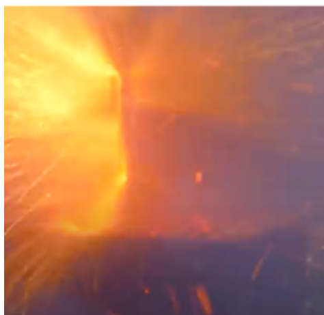
Figure 14: (a) A charged 2.6 Ah cell being deliberately overheated. (b) at the point of rupture (c) the cell takes off as a rocket (d) seconds later the discharge is complete, and the cell is red hot.
