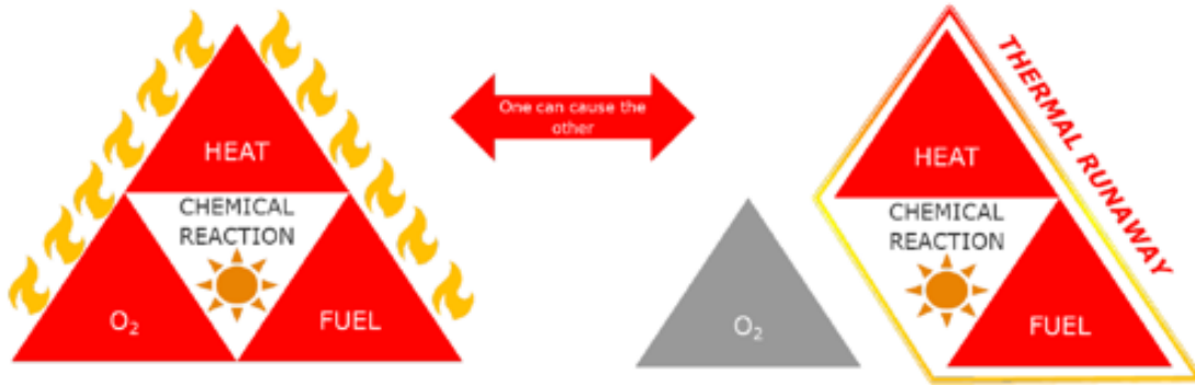
Figure 11 The fire triangle and its relationship to thermal runaway
